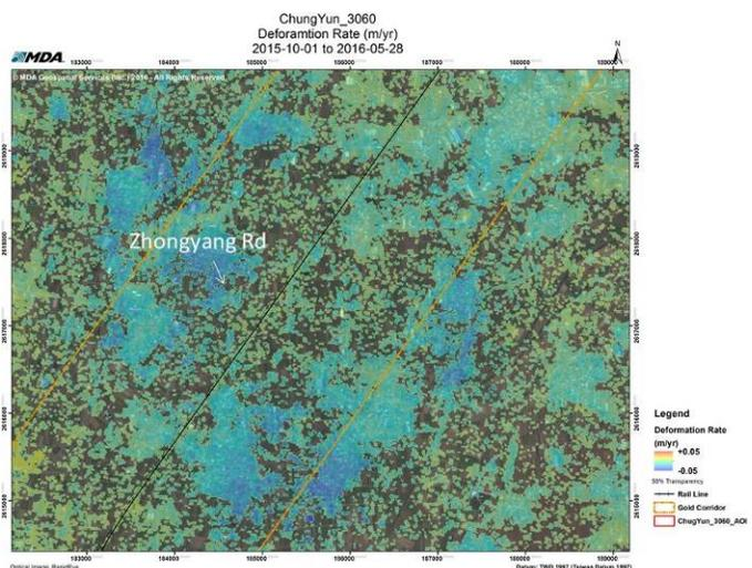
Fig. 7. Deformation rate map in Area 3
