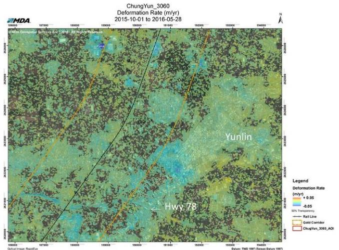
Fig. 6. Deformation rate map in Area 2
