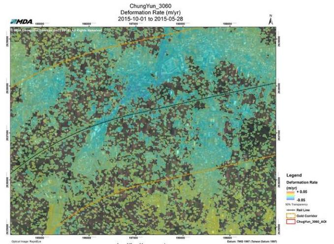
Fig. 5. Deformation rate map in Area 1
