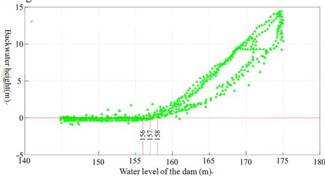
Fig. 2 the influence of water level of the dam on the stage-discharge relationship of Cuntan hydrological station
