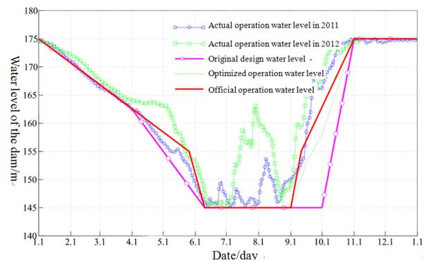
Fig. 1 Three Gorges reservoir water level of the dam operation curve
