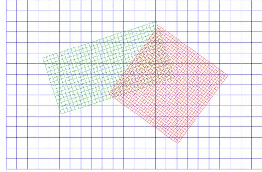
Fig. 1 Schematic of the Chimera grid system. (English et al., 2013)
