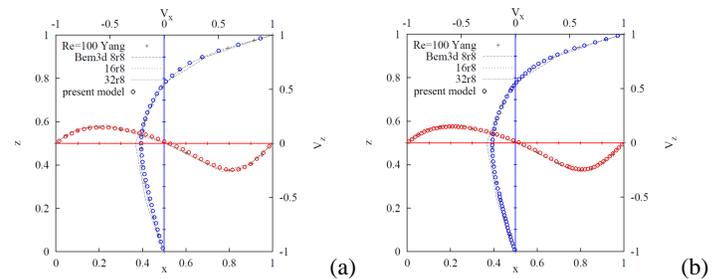
Fig. 2 Velocity profiles along centerlines for  $Re = 100$ . (a) one-block grid system ( $35*35*35$  elements); (b) two-block grid system (the whole:  $70*70*70$  elements, the middle:  $20*20*20$  elements). (+) results of Yang et al. (1998); (-) results of Žunič et al. (2006); and (o) results of present numerical model.
