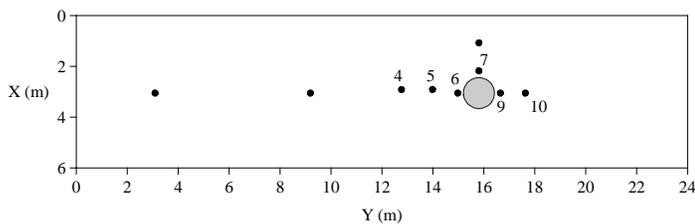
Fig. 3 Sketch of the locations of the cylinder and the wave gauges.
