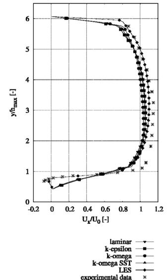
Figure 3. Velocity profiles at  $x_{0.01} = 0.03$  m (end of sill)
