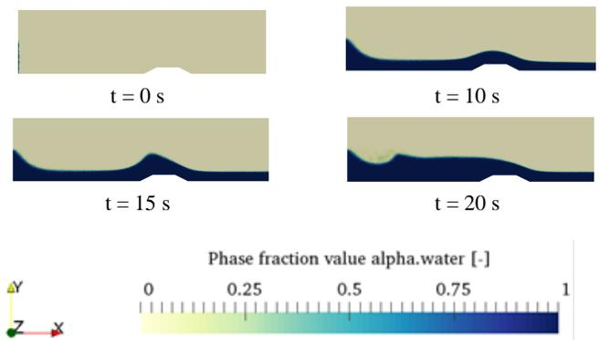
Figure 4. Filling of the domain, segment of the computational domain for different time steps
