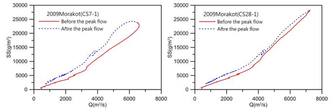
Fig. 7 Suspended load hydrographs during Typhoon Morakot
