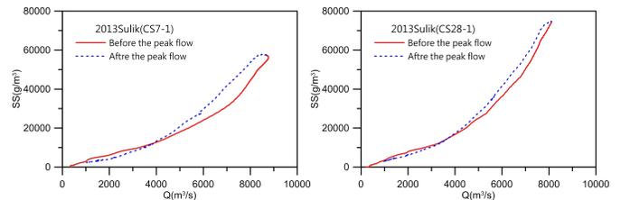
Fig. 8 Suspended load hydrographs during Typhoon Soulik
