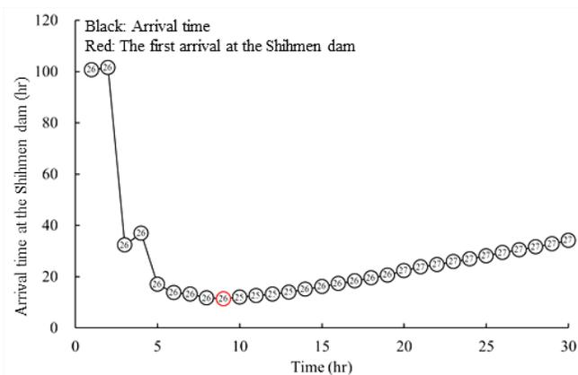
Fig. 8 Plunge point location (the number in the circle means cross section) and arrival time at the Shihmen dam during Typhoon Soulik
