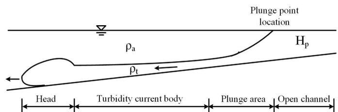
Fig. 1 Sketch of turbidity current plunging
